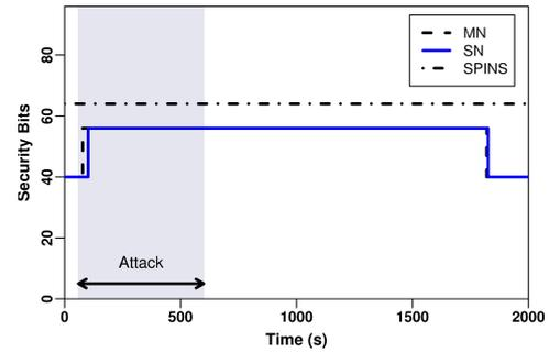
**Fig. 4** HnS’s adaptive security in response to an attack; as the attack begins, MN and SN increase their MAC size.
