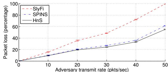
**Fig. 6** Packet loss for different protocols in presence of an adversary. Each point is a mean of 5 trials, with error bars showing 1 standard deviation.
